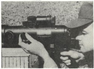
WITHOUT DISTURBING THE LAY OF THE WEAPON OR SCOPE COMBINATION, SIGHT THROUGH THE SCOPE AND BY MANIPULATING THE AZIMUTH KNOB....
