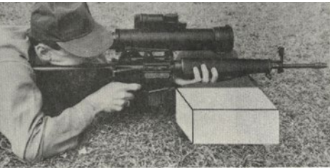
SIGHT THROUGH THE REAR SIGHT OF THE WEAPON (NOT SCOPE) AND ALINE ON THE AIMING POINT OF THE ZERO TARGET
